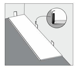
• Use spacers to establish the necessary expansion space between the wall and the perimeter planks, as shown in fig. On the short and long ends of the plank, place spacers with a thickness equal to the required expansion between the plank and the wall. Wait until the installation is finished before removing them. When choosing your starting plank width, remember to account for 5/16" (8 mm) spacing along all walls.
