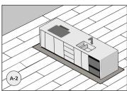
Never obstruct the floor. Heavy objects should be installed first, followed by SPC flooring. Any heavy objects with radiant heat, such as a stove or accumulator, should have a recommended protective plate underneath. As shown in Fig. A1. Therefore, place the heavy item first, as shown in Fig. A2. As it is a floating installation, it should ALWAYS remain buoyant!
