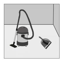
• It is important to make sure that the floor area is always dry, spotless, level, structurally sound, and free of all contaminants (e.g., dust, solvents, grease, chemicals, residual adhesive, adhesive removers, alkaline salts, mold, mildew, debris, etc.) The SPC flooring will feel unsteady and suffer early damage if the subfloor is uneven.
