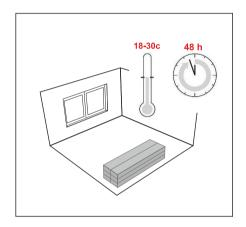
• It is necessary to condition flooring in an environment where temperatures are less than 40°F (5°C) or more than 95°F (35°C), or when relative humidity is less than 35% or more than 70%, by spreading it out in unopened cartons, not stacking, in the room where installation will take place for at least 12 hours in order to achieve the recommended humidity and temperature levels.
